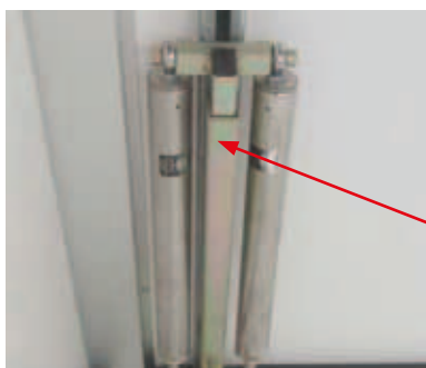
The raising system, using spring-loaded cylinders, is unaffected by temperature. It is guaranteed for 50,000 cycles
